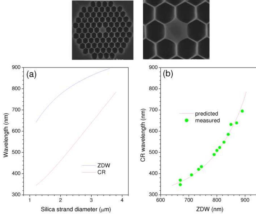
Fig. 1. CR wavelengths associated with 1020 nm pumping. (a) Dependence of the ZDW and the CR wavelength of single silica strand for varying silica strand diameter. (b) Predicted CR wavelength of single silica strand as a function of the ZDW of the silica strand (line), and measured CR wavelengths of 13 high- $\Delta$  PCFs with varying ZDWs (points). Insets: representative scanning electron microscopy images of the cross section (left) and the core (right) of the PCFs.
