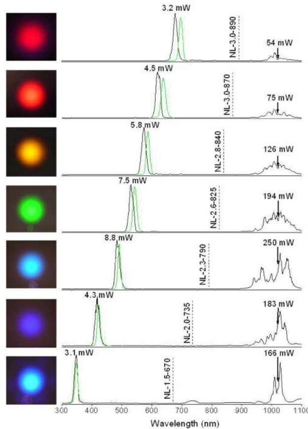
Fig. 2. Dependence of CR spectrum/power of seven high- $\Delta$  PCFs for varying ZDWs (broken vertical lines) and 1020 nm pump powers (arrows). The red-shifted CR spectra (green) are obtained at lower pump powers where the CR signals are minimally observable. The insets show the far-field images of the output light on a paper screen. Autofluorescence from the paper gives the bottom image a false blue color.
