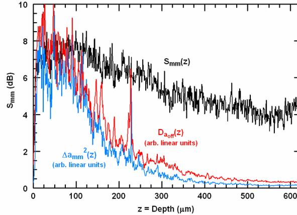
Fig. 7. Depth-dependence of  $\Delta a_{mm}^2$ ,  $D_{aoff}$ , and  $S_{mm}$  for a representative image of a tissue phantom ( $\rho=0.93$  mg/g).  $D_{aoff}$  and  $\Delta a_{mm}^2$  are plotted on a linear scale and are scaled separately for the purposes of comparison (their relative strengths may be determined by  $S_{mm}$ ).
