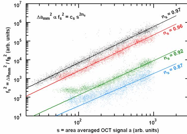
Fig. 6. Scatter plot of  $f_s^2$  versus  $s$  for image sets acquired in tissue phantoms at four concentrations. Black:  $\rho=5.4$  mg/g, red:  $\rho=2.6$  mg/g, green:  $\rho=0.93$  mg/g, and blue:  $\rho=0.45$  mg/g. The associated best fit lines which were fit to data points above the apparent “knee” are drawn.
