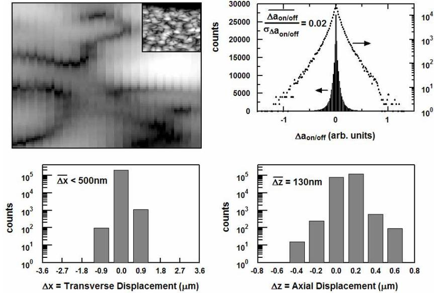
Fig. 2. Mechanics of MMOCT. Upper left: Closeup of MMOCT image ( $20 \times 15 \mu\text{m}$ ) of a tissue phantom ( $\rho=0.93 \text{ mg/g}$ ), inset a larger view ( $110 \times 90 \mu\text{m}$ ). Upper right: Histogram of  $\Delta a_{on/off}$  values from phantom image in linear (left) and log (right) scales as indicated by the arrows. Lower panels: Log histograms of lateral ( $\Delta x$ ) and axial ( $\Delta z$ ) displacements from above image.
