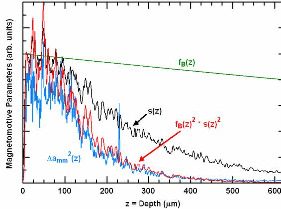
Fig. 5. Depth-dependent functions  $\Delta a_{mm}^2, s, f_B$ , and the  $f_B^2 s^2$  prediction of  $\Delta a_{mm}^2$  are indicated, as averaged laterally across a tissue phantom MMOCT image ( $\rho=0.93$  mg/g). All functions have been scaled separately for the purposes of comparison.
