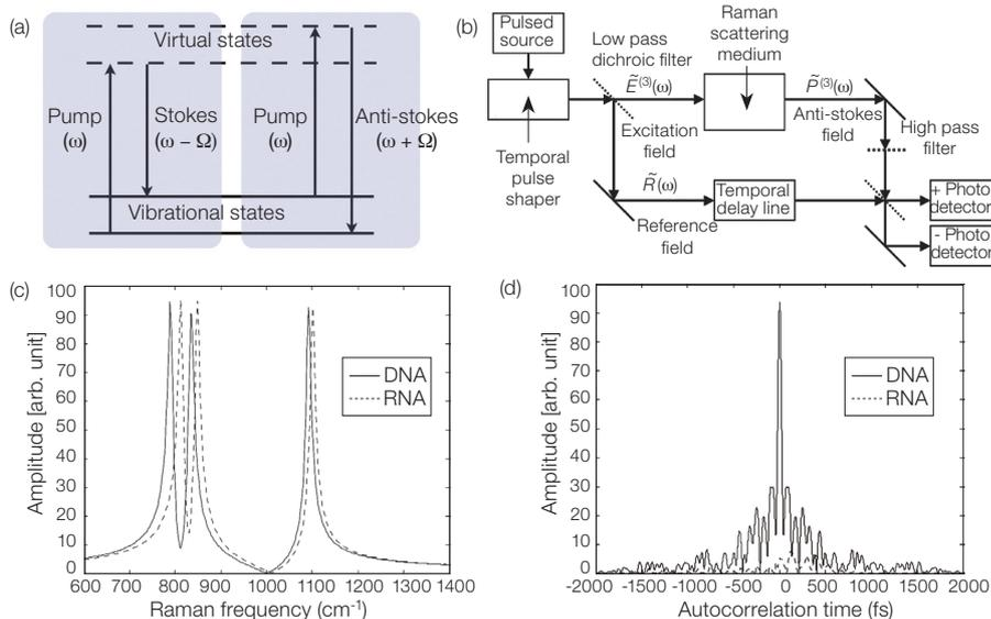
(a) Energy diagram of CARS. (b) Schematic of instrument. (c) Raman spectra of DNA and RNA phosphodiester vibrational modes. (d) Predicted autocorrelation signals from instrument with pulses designed to coherently excite vibrational modes from DNA.
