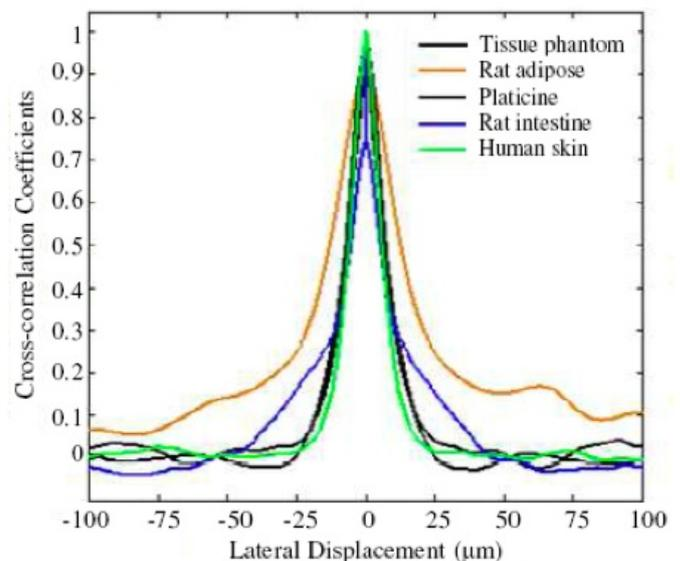
**Figure 1.** Average decorrelation curves obtained from galvanometer-scanned images of several tissue-phantom samples and biological tissues (negative distance corresponds to the cross-correlation between the current and previously acquired A scans). The phantom was a silicone-based sample with titanium dioxide ( $\text{TiO}_2$ )-scattering particles. (Reproduced with permission.<sup>5</sup>)
