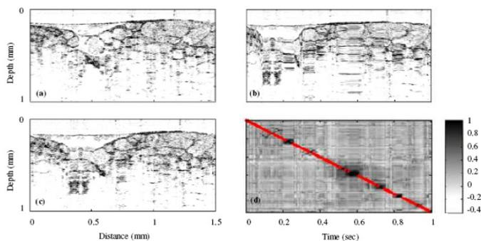
**Figure 2.** Image assembly for human adipose tissue over a sample length of 1.5mm. (a) Galvanometer-scanned image. (b) Nonuniform hand-scanned image. (c) Assembled image. (d) Cross-correlation matrix. Red points show the A scans selected for image assembly. (Reproduced with permission.<sup>5</sup>)
