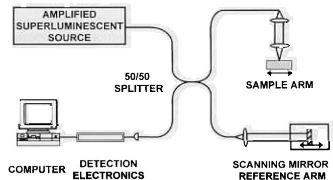
**Fig. 1.** Schematic of the fiber optic implementation of the optical coherence tomography (OCT) system. High-resolution measurements of intensity of backscattered light are performed using a low-coherence length light source and fiber optic interferometer. Two-dimensional cross-sectional images are generated by scanning the light beam in the transverse direction while measuring backscattering intensity versus delay (distance)
