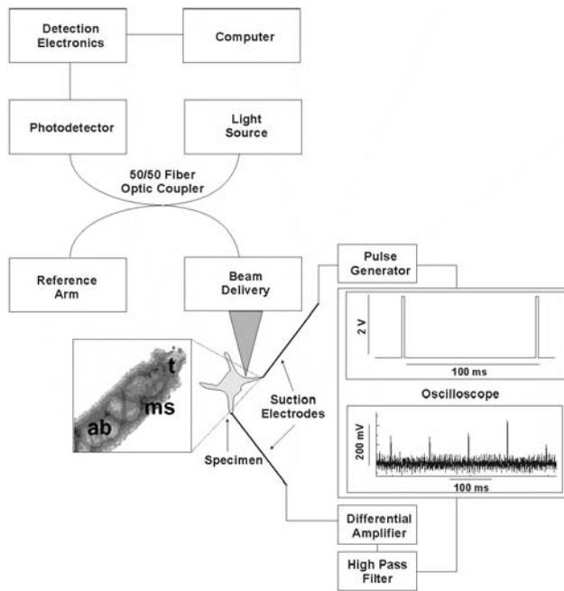
Fig. 1. Experimental setup. The inset shows a light-microscope image of a section of *Aplysia californica* nerve fiber at  $4\times$  magnification. ab, axon bundle; ms, muscle sheath; t, fiber tip.
