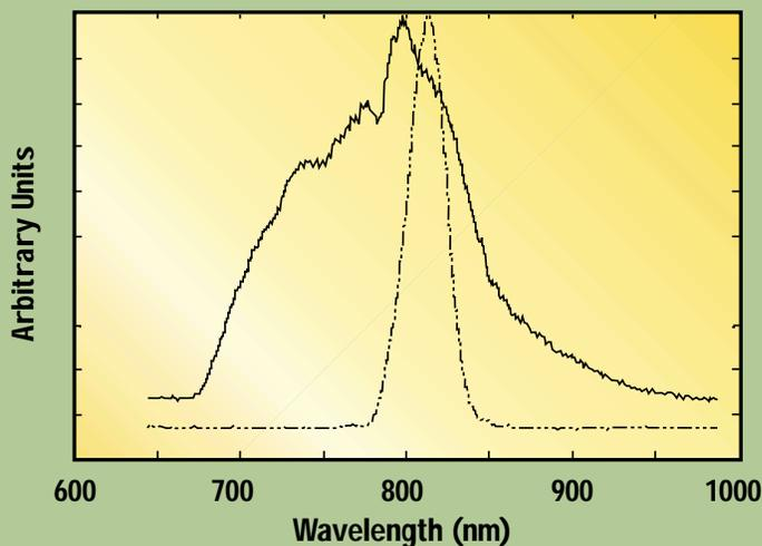
Figure 1 Spectral broadening obtained by pumping high-NA optical fiber with a Ti:sapphire laser can increase OCT imaging resolution.
