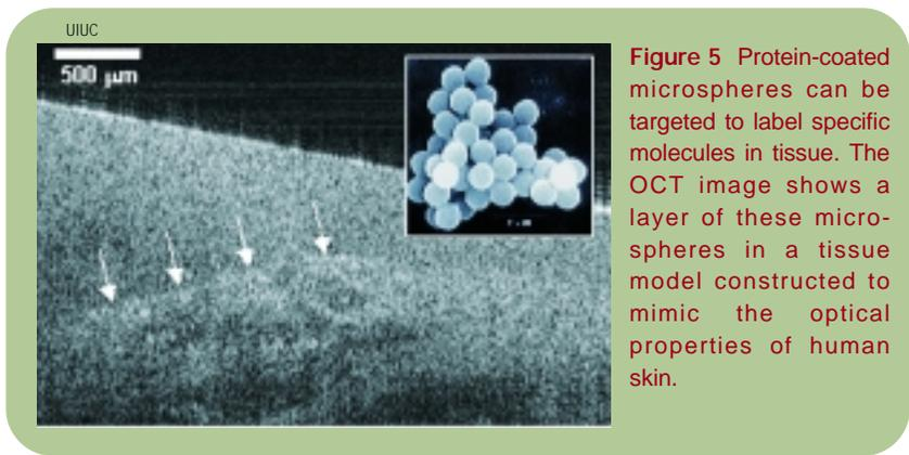
Figure 5 Protein-coated microspheres can be targeted to label specific molecules in tissue. The OCT image shows a layer of these microspheres in a tissue model constructed to mimic the optical properties of human skin.
