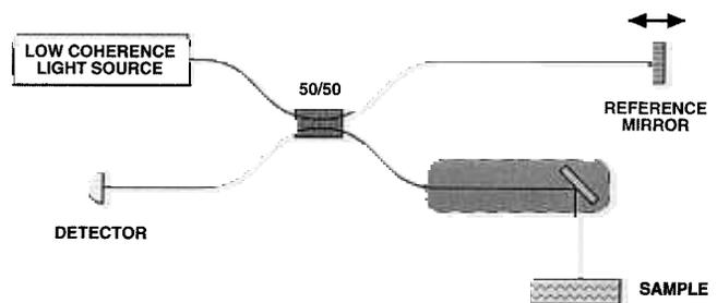
FIG. 1. Schematic of the OCT system. Infrared light generated from the low coherence source is split evenly, half to the sample and half toward a moving mirror. Light is reflected off the reference mirror and from within the sample and recombined in the beam splitter (50/50). The shaded area represents the portion of the system that would be present within the endoscope, consisting primarily of an optical fiber, lens, and mirror.
