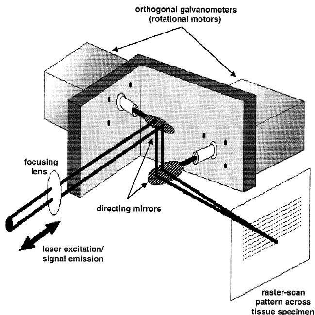
**Fig. 3.** Optical scanning mechanism. Optical imaging techniques may indirectly acquire an image of tissue microstructure by raster-scanning an optical beam across or through the tissue as shown, or by translating the specimen beneath a fixed optical beam. One example is laser-scanning confocal microscopy, which produces images based on the optical intensity at each pixel.
