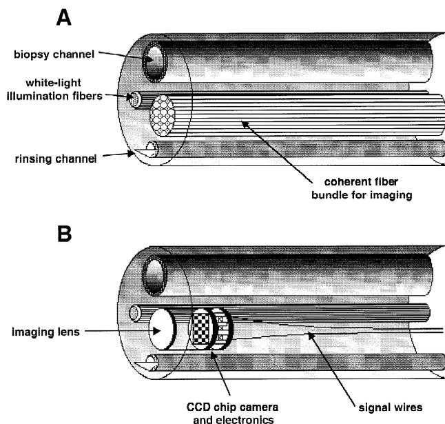
**Fig. 2.** Flexible endoscope optical elements. **A** Coherent fiber-optic imaging bundle used to relay image of tissue. **B** A single miniature CCD (charge-coupled device) camera can be located at the tip of a flexible endoscope. Images are digitized and converted to electrical signals for transmission to the proximal end, where the digital image is displayed on a video monitor.
